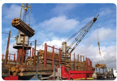
Logs transferred from truck to ship with use of the ships gear by Associated Terminals of St. Bernard team members.
